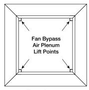
Top view of **Bypass Air Plenum**
